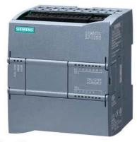
SIMATIC S7-1200, CPU 1212C, compact CPU, AC/DC/relay, onboard I/O: 8 DI 24 V DC; 6 DO relay 2 A; 2 AI 0-10 V DC, Power supply: AC 85-264 V AC at 47-63 Hz, Program/data memory 75 KB
