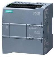
SIMATIC S7-1200, CPU 1212C, compact CPU, DC/DC/DC, onboard I/O: 8 DI 24 V DC; 6 DO 24 V DC; 2 AI 0-10 V DC, Power supply: DC 20.4-28.8V DC, Program/data memory 75 KB
