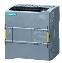
SIMATIC S7-1200F, CPU 1212 FC, compact CPU, DC/DC/DC, onboard I/O: 8 DI 24 V DC; 6 DO 24 V DC; 2 AI 0-10 V DC, Power supply: DC 20.4-28.8V DC, Program/data memory 100 KB
