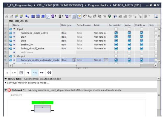
® This determines that the #Conveyor\_motor\_automatic\_mode parameter is written by this block. Still missing, however, are the input conditions so that this actually happens. An SR flip-flop and #Enable\_OK parameter are logically combined with an AND logic operation at the input of the assignment block. To do this, first click the input of the block so that the input line has a blue background.
