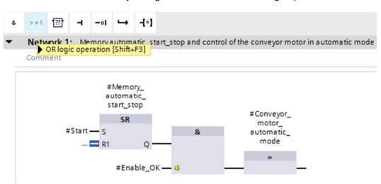
® The OR block has 2 inputs initially. In order to logically combine an additional input tag, click the yellow star
