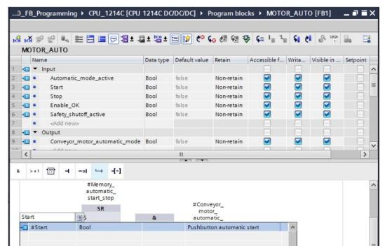
**Note:** When assigning tags in this way, there is a risk of a mix-up with the global tags from the tag table. The previously presented procedure using drag & drop from the interface description should therefore be used preferentially.
