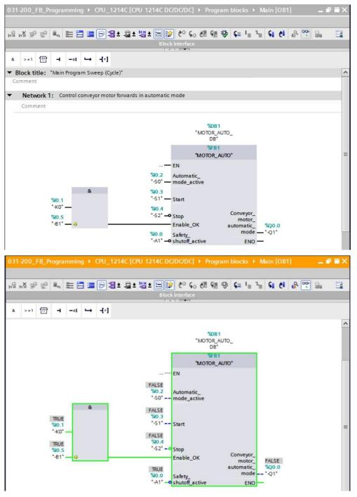
**Note:** The monitoring here is signal-related and controller-dependent. The signal states at the terminals are indicated with TRUE or FALSE.
