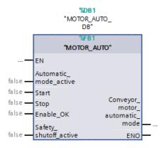
® To insert an AND before input parameter "Enable\_OK", select this input and insert the AND by clicking the icon in your logic toolbar (® ).
