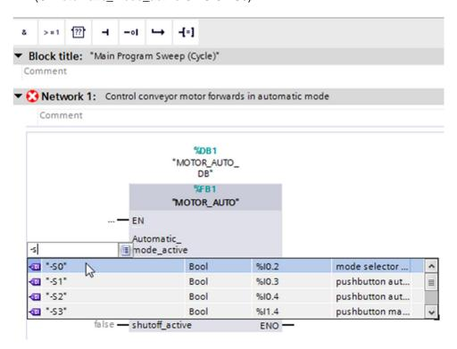
Insert the other input tags "-S1", "-S2", "-K0", "-B1" and "-A1" and then insert output tag "-Q1" (%Q0.0) at output "Conveyor\_motor\_automatic\_mode".
