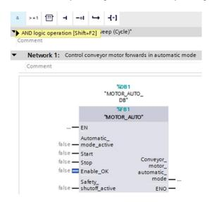
® To connect the block to the global tags from "Tag\_table\_sorting\_station", we have two options:
