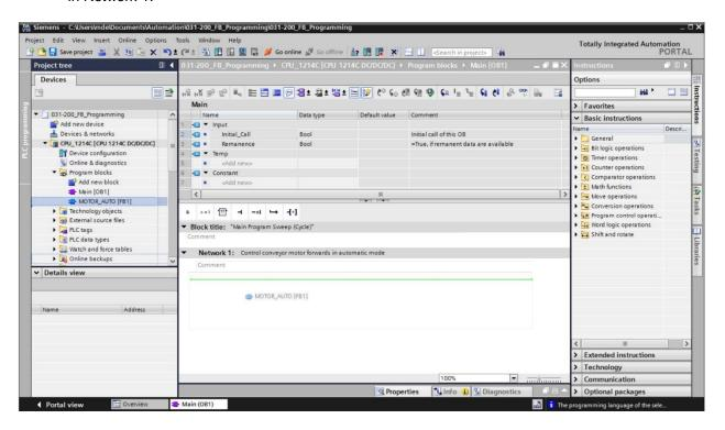
® The instance data block for this call of FB1 is created automatically. Assign a name and apply it with OK. (® MOTOR\_AUTO\_DB1 ® OK)
