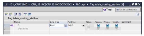
® Change the address to %Q0.0 (Q 0.0) by entering this directly or by clicking the drop-down arrow to open the Addressing menu. Change the operand identifier to Q and confirm with Enter or by clicking the check mark (® %I0.0 ® Operand identifier® Q ® ✓ )
