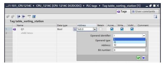
® Enter the "Conveyor motor M1 forwards fixed speed" comment for the tag.
