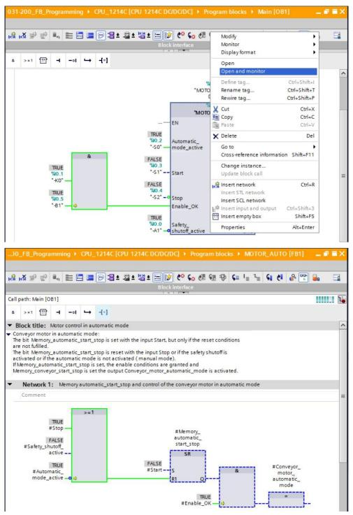
**Note:** The monitoring here is function-related and controller-independent. The actuation of sensors and the station status are shown here with TRUE or FALSE.
