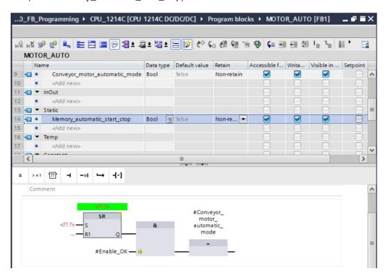
® The #Memory\_automatic\_start\_stop will be set with input tag #Start. Click twice on the S input of the SR flip-flop <??.?> and enter "Start" in the field that appears in order to see a list of available tags starting with "Start".Click the #Start tag and apply with ® Enter.
