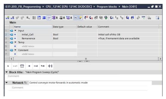
® Use drag & drop to move your "MOTOR\_AUTO [FB1]" function block onto the green line in Network 1.
