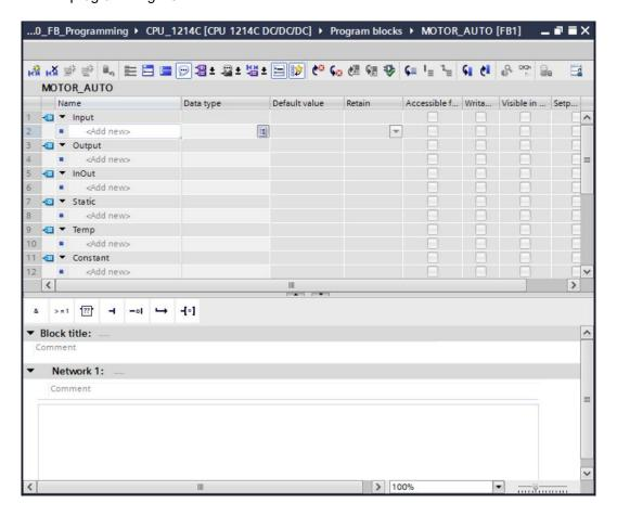
A binary output signal is needed for controlling the conveyor motor. For this reason, we first create local output tag #Conveyor\_motor\_automatic\_mode of the "Bool" type. Enter the comment "Control of the conveyor motor in automatic mode" for the parameter.
