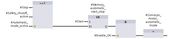
® Negate the input connected to parameter #Automatic\_mode\_active by selecting it and clicking
