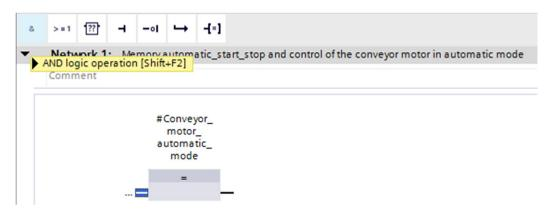
® Use drag & drop to move input parameter #Enable\_OK onto the second input of the & logic operation <??.?>. (® < Enable\_OK)</p>
