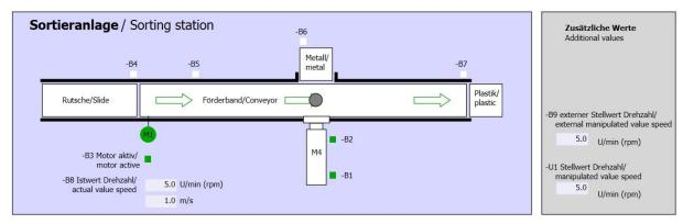
Figure 8: Technology diagram
