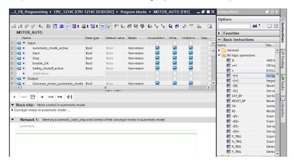
Now use drag & drop to move your output parameter #Conveyor\_motor\_automatic\_mode onto <??.?> above the block you just inserted. The best way to select a parameter in the interface description is by "grabbing" it at the blue symbol . (® Conveyor\_motor\_automatic\_mode)
