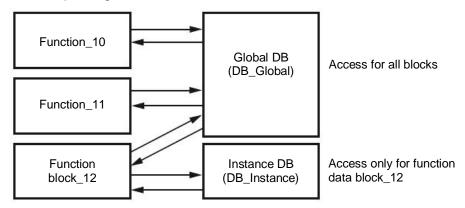
Figure 5: Difference between global DB and instance DB.
